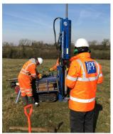
Although the site was agricultural fields at the time of the investigation, areas of deep made ground associated with the coal mining was identified and associated contamination testing associated with the former site usages was undertaken.
